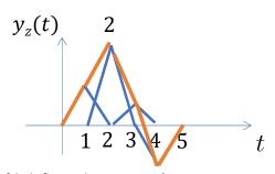
Since the system is LTI we found output  $y_z(t)$  only with this information: -1  $x_1(t)$   $x_1(t)$   $x_1(t)$   $x_2(t) = 2x_1(t-1)$   $x_2(t) = 2x_1(t-1)$   $x_3(t) = 0.5x_1(t-2)$   $x_3(t) = 0.5x_1(t-2)$
