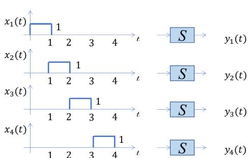
Can we find  $y_2(t)$  and  $y_3(t)$  and  $y_4(t)$  only by using the available  $y_1(t)$ ? Only if the system is also TI!
