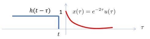
2- For t>0 there is a partial overlap, and the convolution is equal to the area under the overlapped section.
