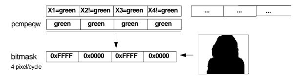
This mask is now used on the same four pixels from the picture with the woman and the equivalent four pixels from the Spring blossom. The "AND NOT" and "AND" instructions use the mask to identify which pixels to keep from the Spring blossom and the woman. They also turn the unwanted pixels to zeros. The "OR" instruction builds the final picture. Four pixels were mapped using only four MMX instructions without any branches.
