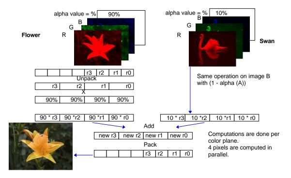
If these images use 640X480 resolution, and the dissolve technique uses all 255 steps of the alpha value, then 117 million PUNPCKs and PMULs, and 58 million PADDs and PACKs are used. Comparing instruction counts with and without MMX technology for this operation yields the following:
