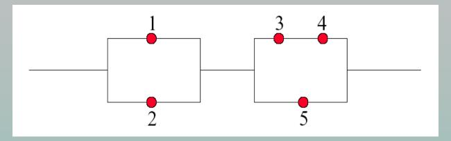
Total reliability is the reliability of the first half, in serial with the second half. Given R1=0.9, R2=0.9, R3=0.99, R4=0.99, R5=0.87
