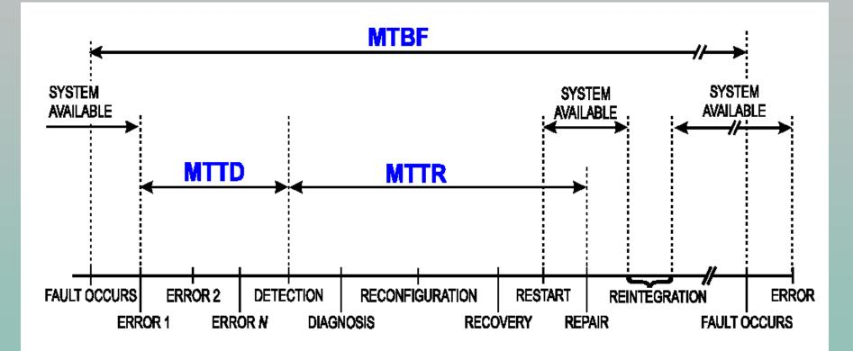
A Scenario for on-line detection and off-line repair. The measures – MTBF, MTTD, and MTTR are the average times to failure, to detection, and to repair.
