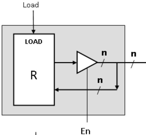
**Tri-state bus using bi-directional lines.**
