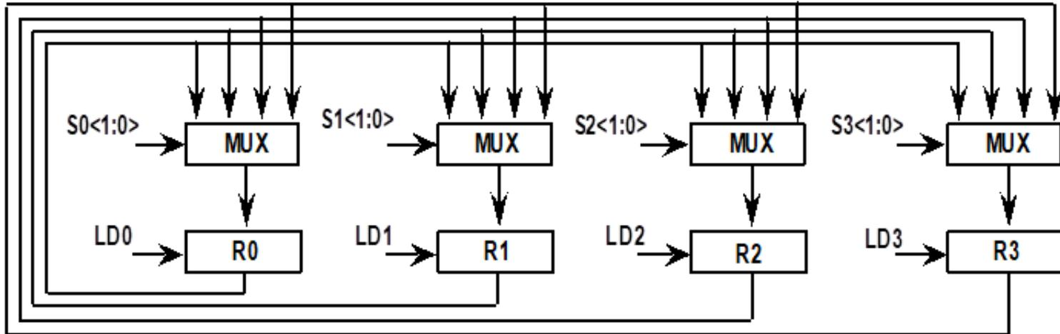
Modules have edge-triggered N-bit registers to transfer, controlled by  $LD_i$  signals.
