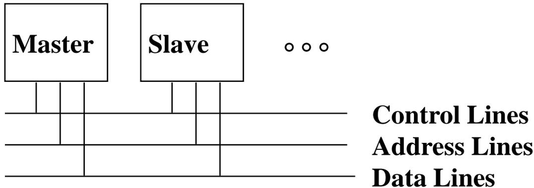
**Bus Master:** has ability to control the bus, initiates transaction
