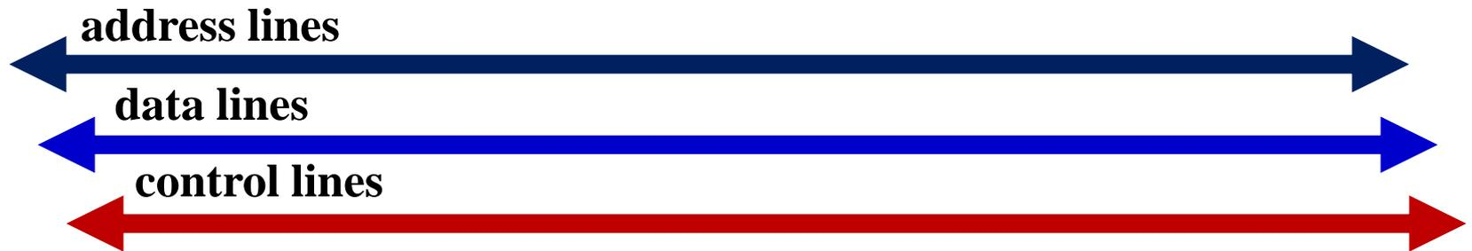
**Typically a bus has three types of signal lines**
