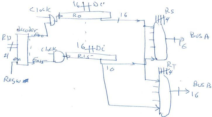
Q2-2 Explain how a READ operations from Register 7, and Register 9 can be performed at the same time
