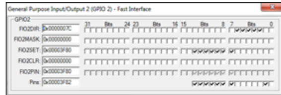
Figure 18: GPIO Peripheral Window
