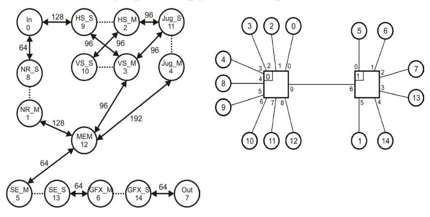
• The optimal Application-specific NoC has two routers with 10 and 7 ports.
