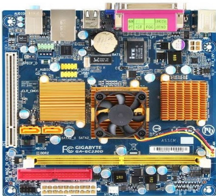
PC Motherboard – CPU with support ICs
