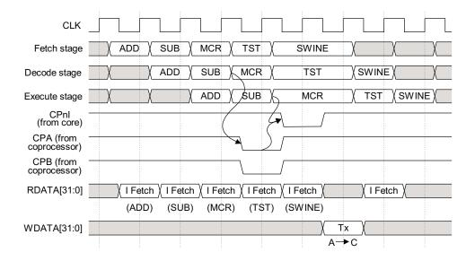
Figure 4-2 Coprocessor register transfer sequence
