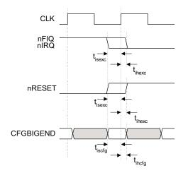
Figure 8-3 Exception and configuration input timing
