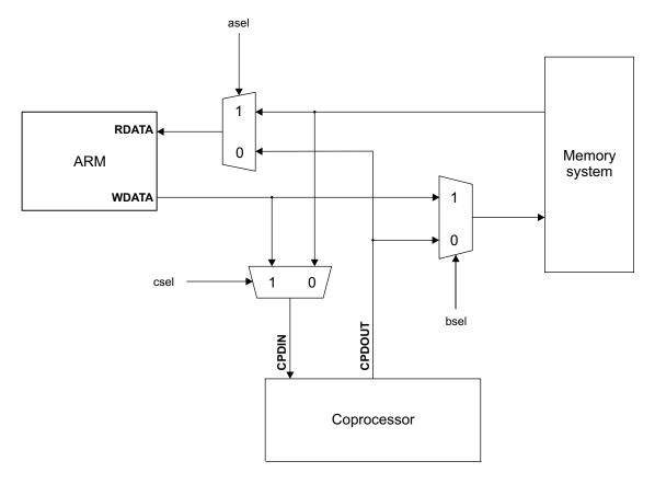
Figure 4-5 Coprocessor connections
