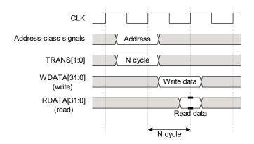
Figure 3-2 Nonsequential memory cycle
