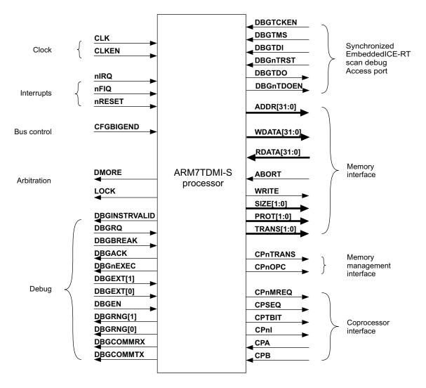
Figure 1-4 ARM7TDMI-S functional diagram
