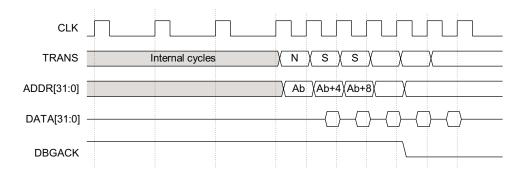
Figure 5-11 Debug exit sequence
