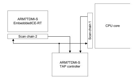
Figure 5-7 ARM7TDMI-S scan chain arrangements
