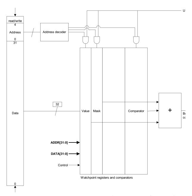
Figure 5-12 EmbeddedICE-RT block diagram
