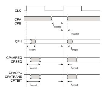
Figure 8-2 Coprocessor timing
