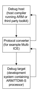
Figure 5-1 Typical debug system
