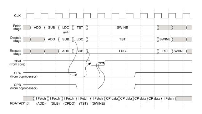
Figure 4-4 Coprocessor load sequence
