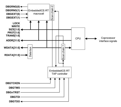
Figure 1-2 ARM7TDMI-S block diagram
