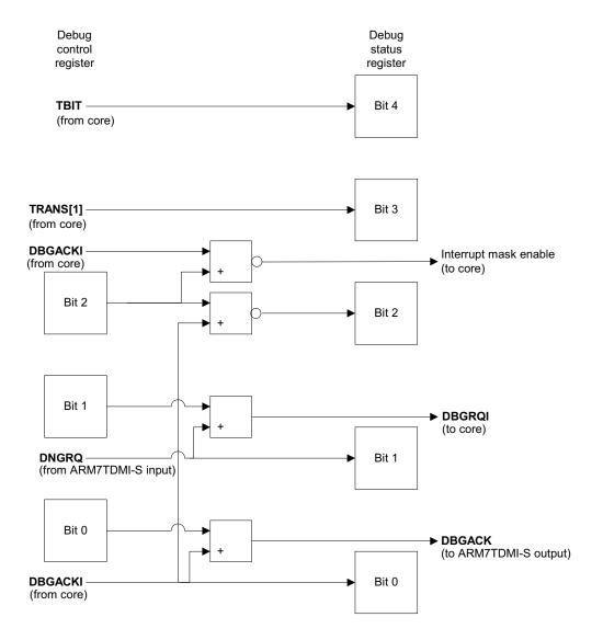
Figure 5-17 Debug control and status register structure
