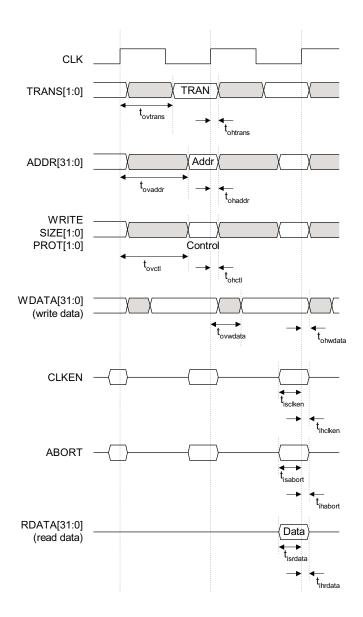
Figure 8-1 Timing parameters for data accesses
