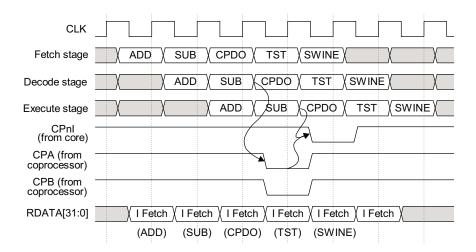
Figure 4-3 Coprocessor data operation sequence
