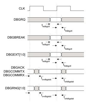
Figure 8-4 Debug timing
