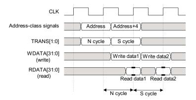
Figure 3-4 Sequential access cycles
