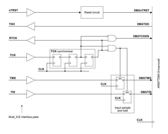
Figure 5-4 Clock synchronization
