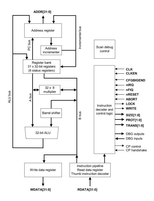
Figure 1-3 ARM7TDMI-S core
